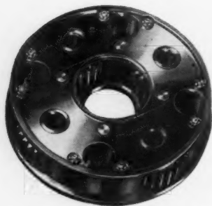
Main rotor drive built by Foote Bros. for use on Piasecki Helicopters
